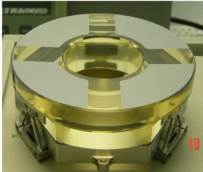
Figure 6. EUVI primary mirror, coated and mounted. the mirror diameter is 105 mm. The regions between the quadrants are deliberately left uncoated.
